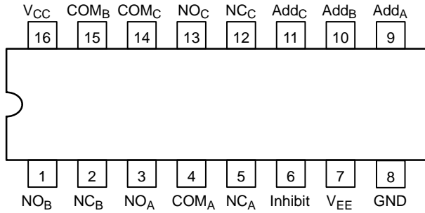
Figure 1. Pin Connection (Top View)
